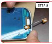
Be careful and remember to pull the menu button flex cable through the bottom.
