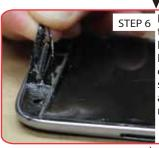
Remove the old adhesive from the inside of the phone and LCD. We recommend using Isopropyl Alcohol and a fine clean cloth. If possible save 2 small pieces of the old LCD adhesive. They will be helpful in reattaching the menu buttons later.
