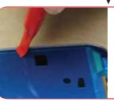
Use the back of the plastic prytool included in your kit to press the adhesive into the phone firmly. A tight fit is important for holding the menu buttons back in place.
