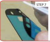
Remove the clear backing from the ProKit Adhesive and place exposed adhesive gasket into the outline of the phone.
