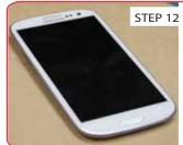
STEP 12 Press new glass into place, no further heating is required.
